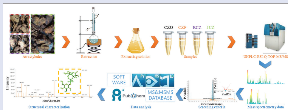
Figure 1: Experimental procedures for composition analysis of different processed products from Atractylodes Rhizome based on UHPLC-Q-TOF-MS/MS
